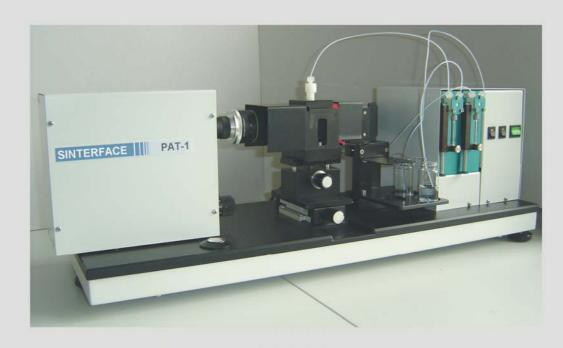
Most modern method to measure the surface and interfacial tension of liquids
