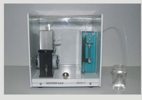
Classical method to measure the surface and interfacial tension of liquids
