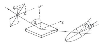
The change in the state of polarization is the direct consequence of interference within the layer system. It is captured by the so called ellipsometric angles  $\Delta$  and  $\Psi$ .
