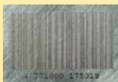
Marking of stainless steel
