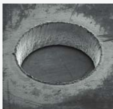
Hole made in 200 µm thickness stainless steel: Inlet, diameter 570 µm Outlet, diameter 475 µm
