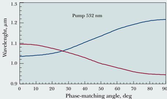
Fig. 3. OPO tuning curve in x-y plane
