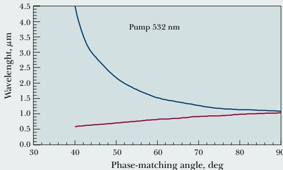
Fig. 4. OPO tuning curve in x-z plane
