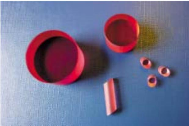
$\text{Al}_2\text{O}_3:\text{Ti}^{3+}$  – titanium-doped sapphire crystals combine supreme physical and optical properties with broadest lasing range.
