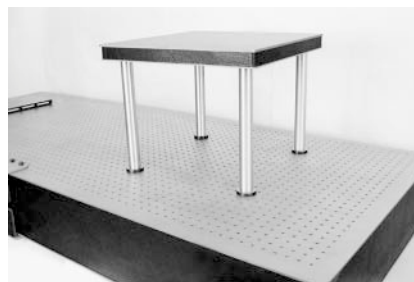
A breadboard may be mounted on a table by silent rods
